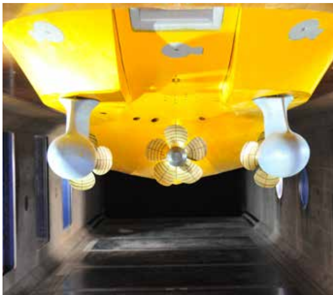
A ship model undergoing testing at HSVA
