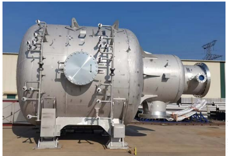
The Cluster 5 Double Layer has a diameter of 3,900 mm and a total weight of 28 metric tons
