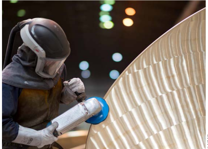
The propeller is given the finishing touches after casting
