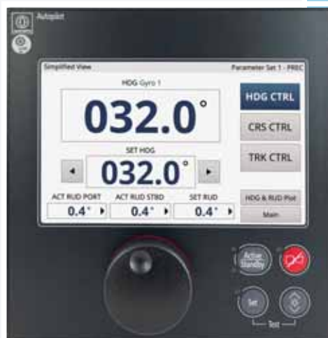
The »Toe Angle« function helps to save fuel, especially on vessels with twin rudders
