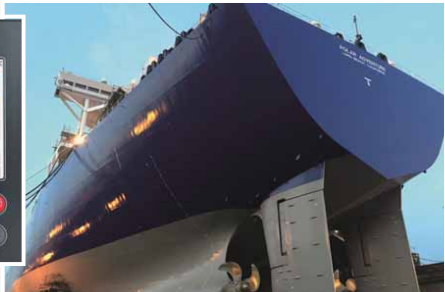
The »Toe Angle« function helps to save fuel, especially on vessels with twin rudders
