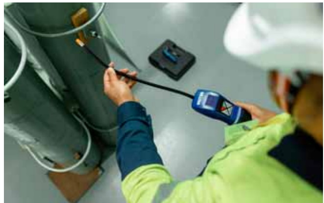
A handheld detector able to detect all halogen refrigerants (CFC, HCFC, HFC, HFO), enabling the detection of leaks in refrigeration systems and minimizing refrigerant loss
