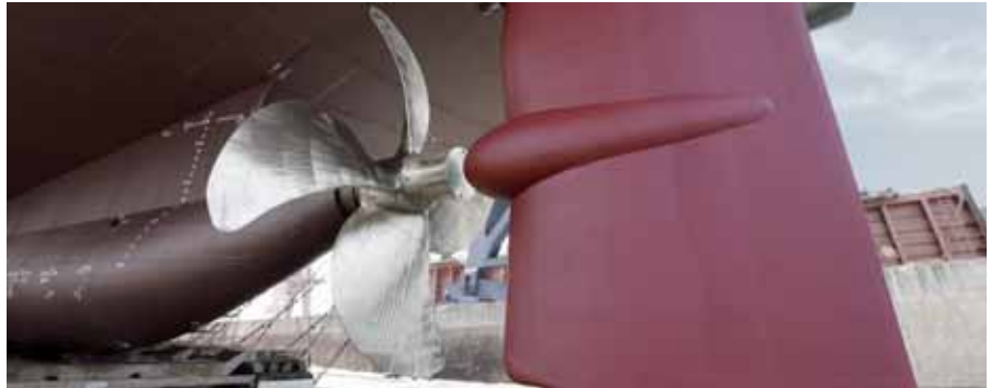
Damen's ESPAC rudder efficiently directs turbulent water along the rudder blade
