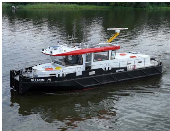
© WSA The »Mülheim« runs completely on battery power
