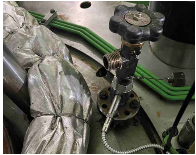
TCS-01CA-PMI sensor installed on a MAN 6S60 ME two-stroke engine
